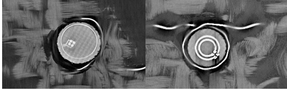
X-ray computed tomography images of embedded tags
