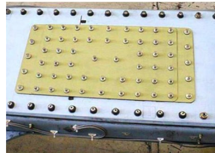
Figure 1: Repair by riveted plate
